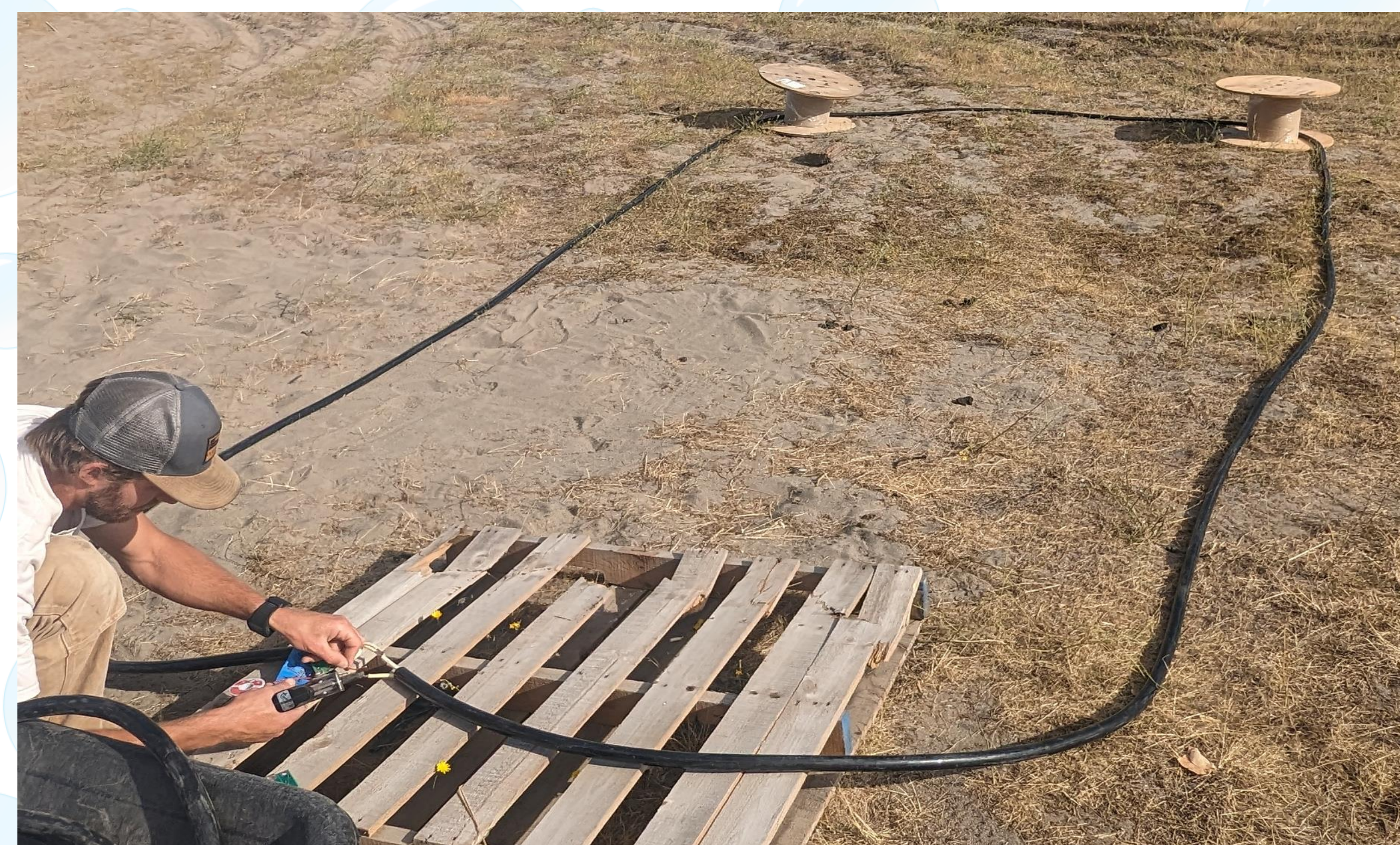
Purged antennas are evaluated for current, signal noise, capacitance and read range prior to re-deployment. If parameters do not meet criteria, antennas are placed in direct sun to heat up or "bake." Repeated purging and baking cycles improved function in cable with deep water intrusion.
